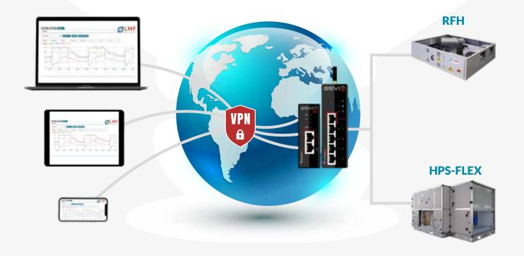
The Sevio LMF system uses a secure communication protocol thanks to the use of a VPN (virtual private network). VPNs use links that require authentication to ensure that only authorised users may access them using encryption systems.
